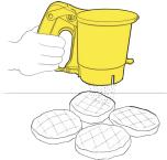
Place unit over targeted area, squeeze handle and release
